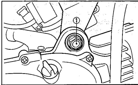
6. Remove the spark plug cap.
