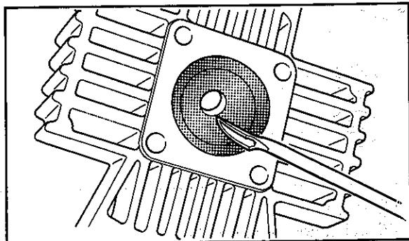
After cleaning the cylinder head, inspect it for damage. If there is any damage, such as cracks or holes, it must be repaired or replaced. If the head is warped, it may need to be resurfaced. This process involves removing a thin layer of metal from the head to correct any warpage. It is important to use the correct grit size of sandpaper and follow a specific sanding pattern to avoid removing too much material from one side of the head.
