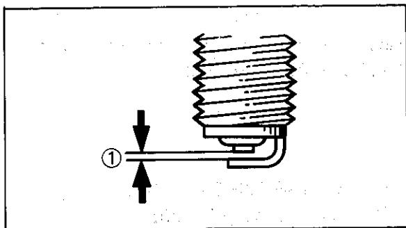
1. Measure the electrode gap ① with a wire thickness gauge.
